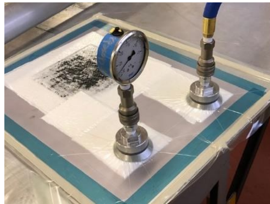
Figure 5.1 Infusion process of CFRP matrix composite laminate fabrication
